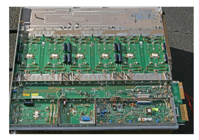
Well designed TV surplus amplifier with many conversion options for use on 222 MHz.
